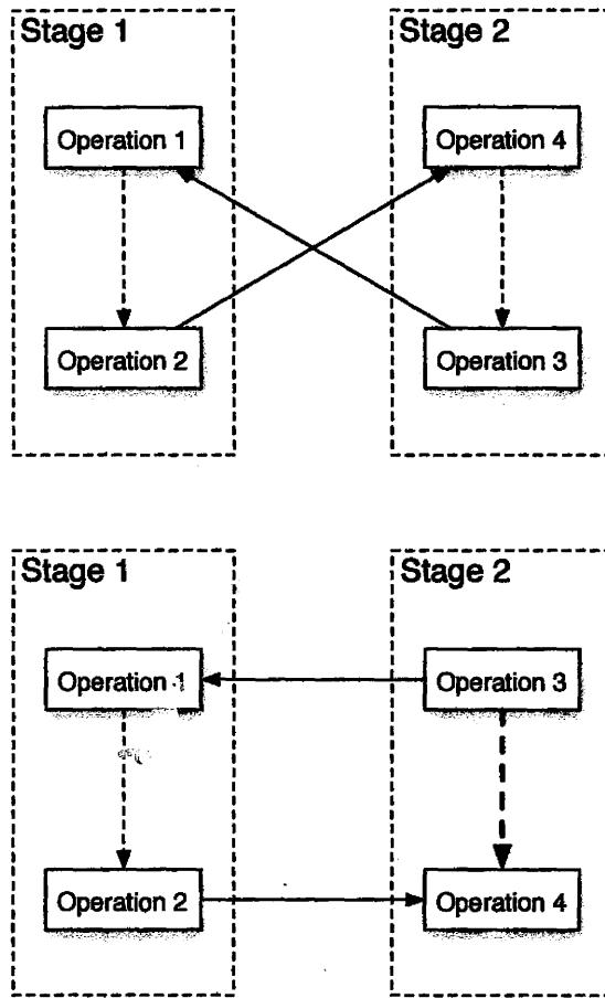
Figure 5.1: Avoiding dependence cycles when scheduling separately
