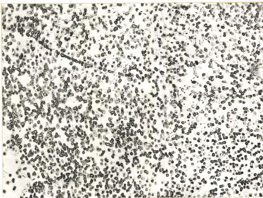
Fig. 33 Mechanically polished sample etched in hydrogen X 170.
