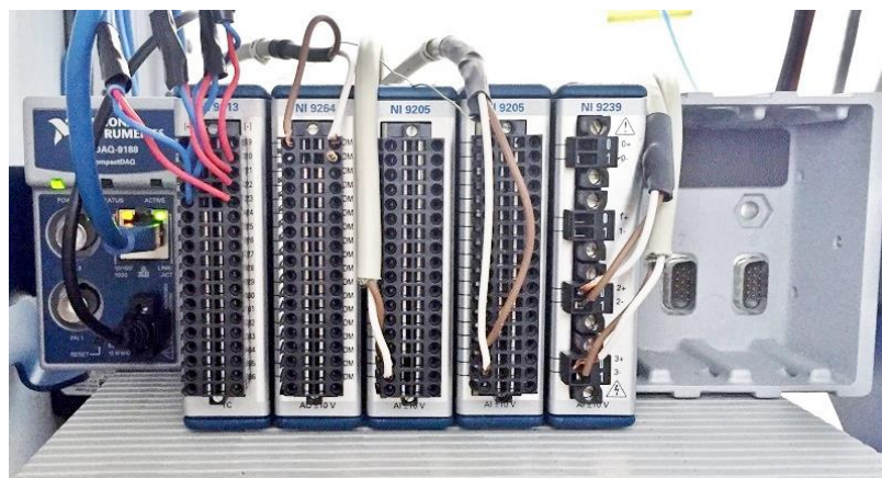
Figure 4.21. The data acquisition module that captures and logs the signals for further analysis
