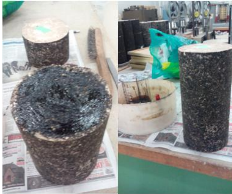
Figure 3.5.2: FASB Specimen bonding for cyclic triaxial testing
