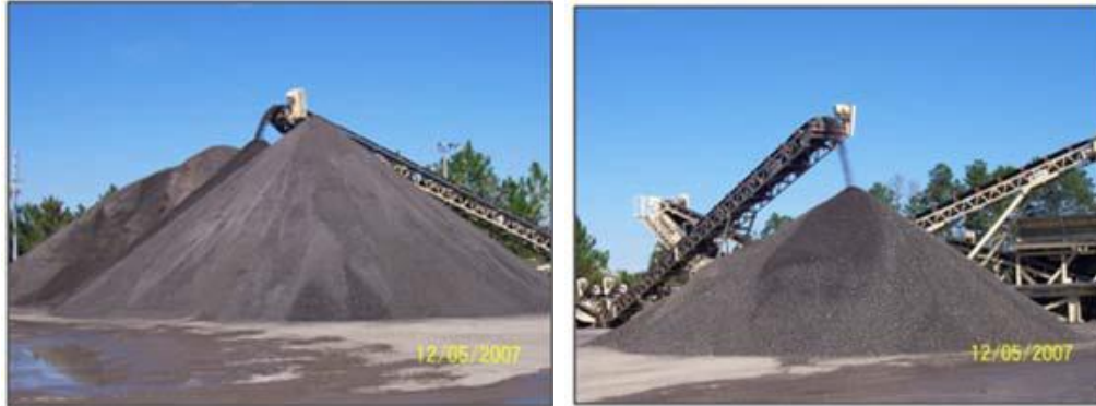
Figure 2.4.1: Fine (left) and coarse (right) fractionated RAP[2]
