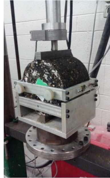
Figure 3.4.1: Indirect tension test setup with LVDT's for measuring horizontal displacements used in IDT Mr testing
