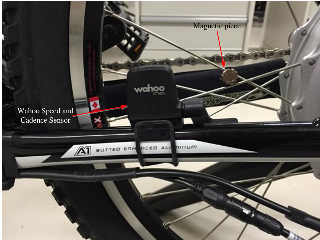
Figure 3.2 The Wahoo speed and cadence sensor with magnetic piece
