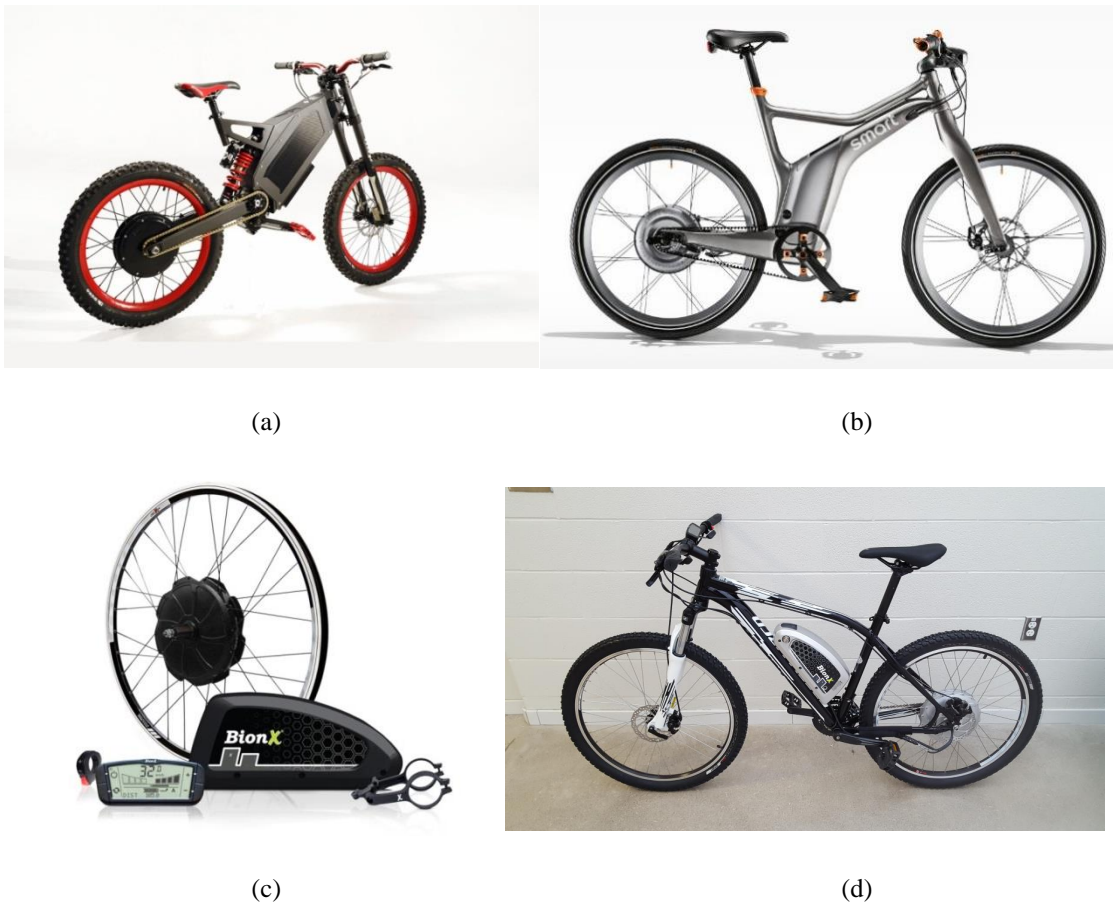
Figure 1.1 Some examples of commercial E-bicycles: (a) Stealth Electric Bikes B-52, with maximum 5.2 kW motor output, up to 80 km/h and 80 km range, (b) Smart Electric Bicycle powered by BionX motor, battery and control unit, (c) BionX conversion kit (48 V, 8.8 Ah battery pack and 350 W motor), and (d) Electrified bike by BionX conversion kit
