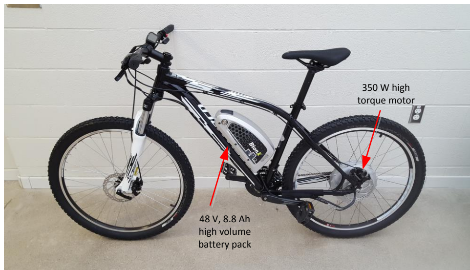
Figure 3.1 Electrified bike using BionX conversion kit
