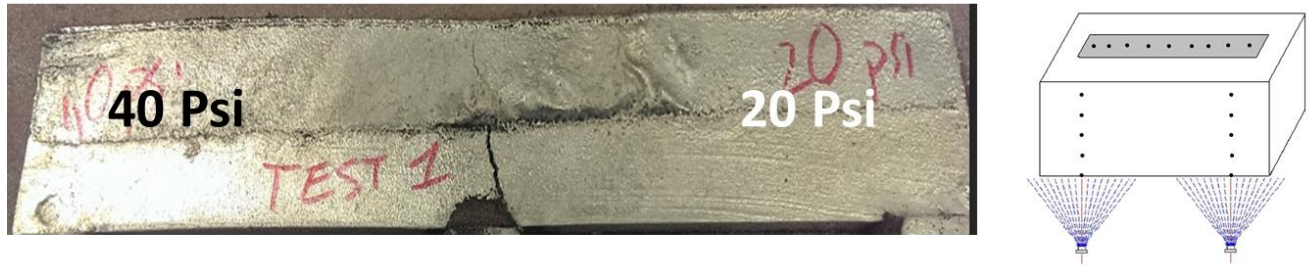
Figure 17: Crack formation due to the meeting of two solidification fronts in the case of two HiPerMag jets (note: numbers on the plate show the regional pressures)
