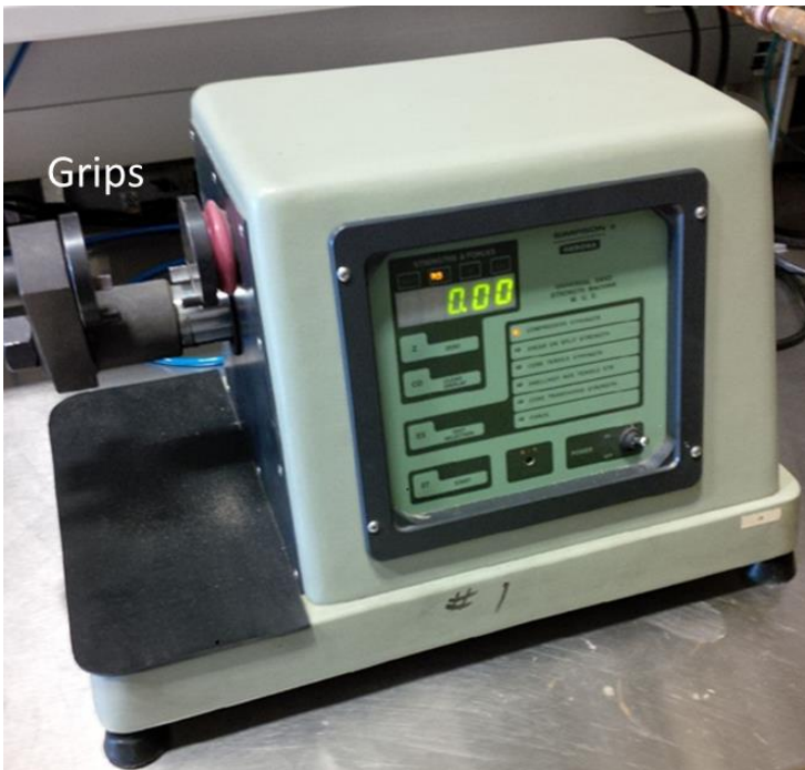
Figure 24: Universal sand testing machine showing grips for the compression test samples
