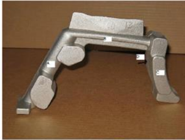
Figure 10: The military handle casting after Tiryakioglu et al. [20], showing the locations from which the specimens were excised
