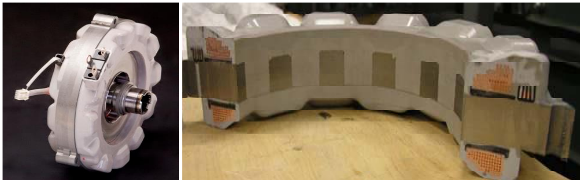
Fig. 2.9. Toyota Prius 2010 generator and its stator cross section [59].
