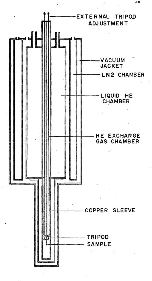
tripod within the cryostat. They could then be aligned to greater precision using the neutron beam. A further adjustment was necessary after the samples were cooled due to differential thermal expansion of the sample holder.
