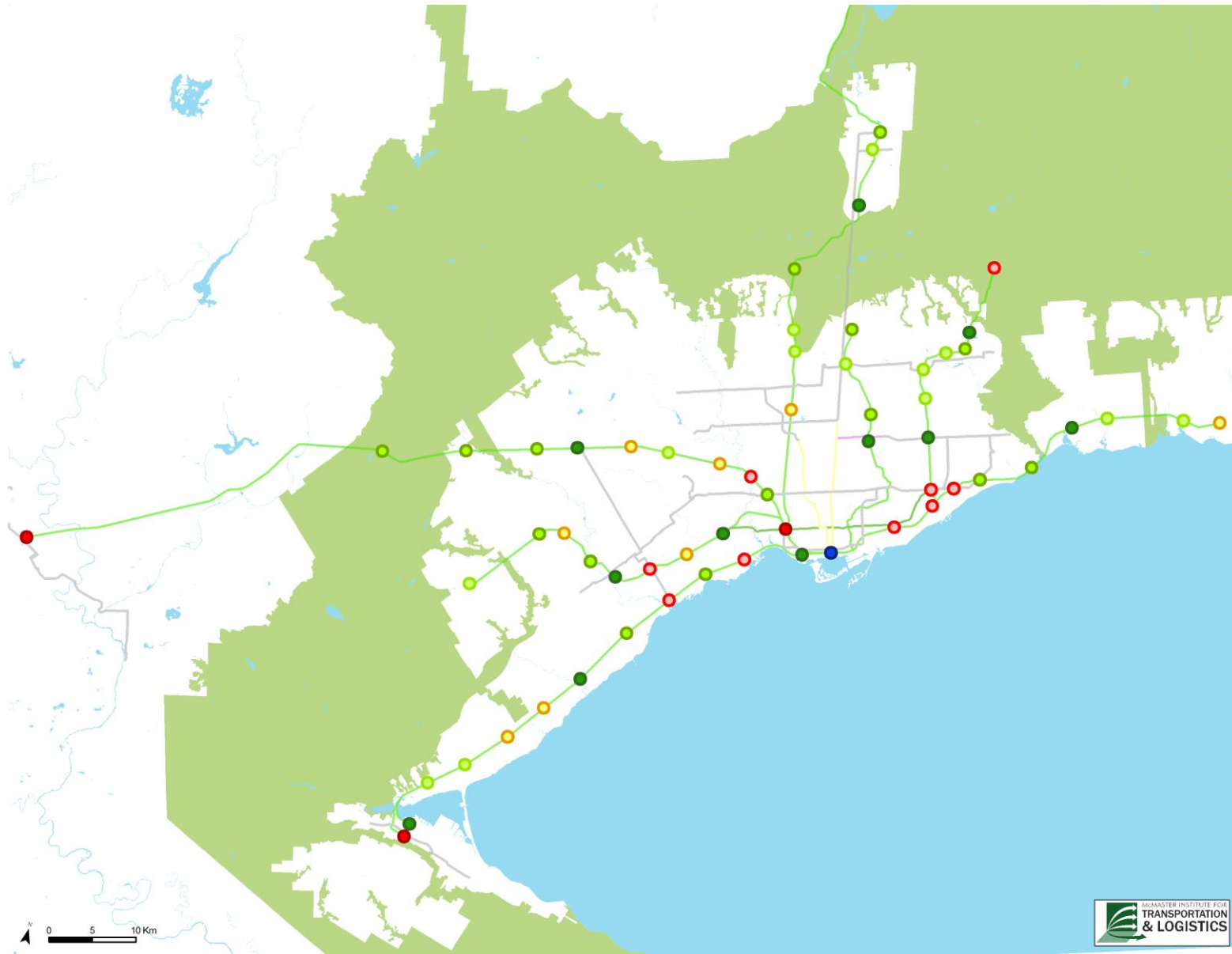
Figure 3-42. Station Designations on the GO CRT Network
