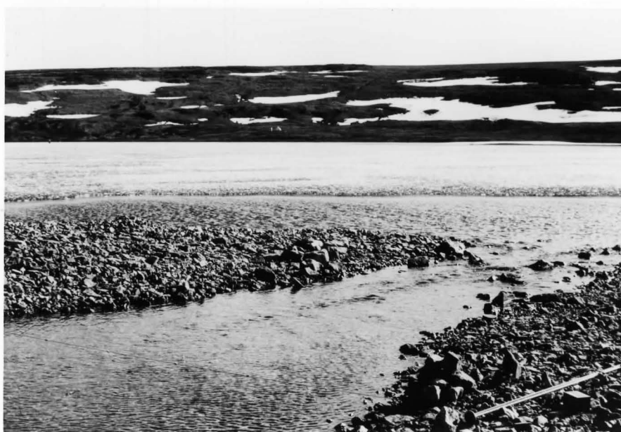
Figure 2.7 The outflow channel at the southwestern end of Three Mile Lake . Top: During the snowmelt period before the channel-break. Bottom: After the channel-break but still early in the season. Note the rope knotted at 0.5 m. intervals across the channel. A wading rod and current meter are at the lower right of the photo.
