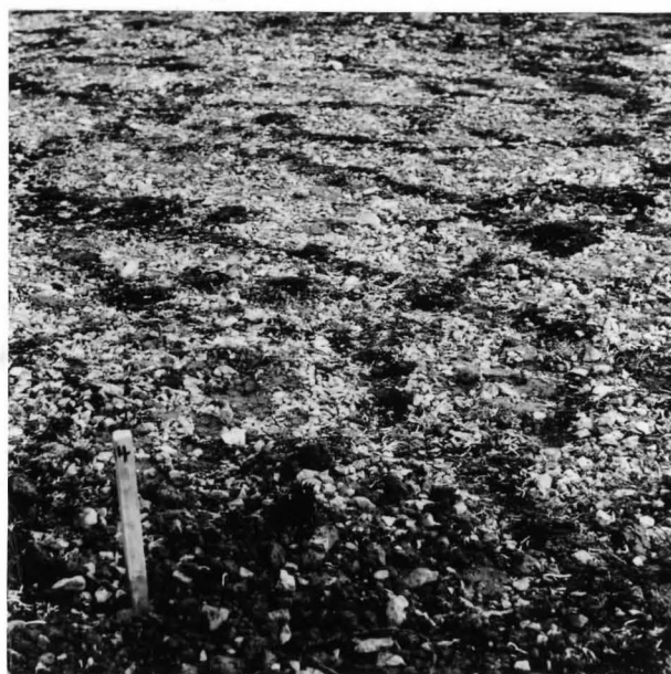
Figure 2.5 Evaporation lysimeters in an area east of Three Mile Lake : the top photo shows the 'dry bog' lysimeter; the bottom photo a 'wet gravel' lysimeter.
