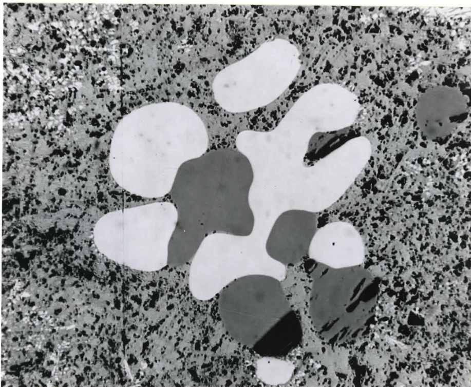
Figure 5.7 Three-phase ( \gamma -Fe + MnS + FeS) equilibrium. at 1190°C. X225
