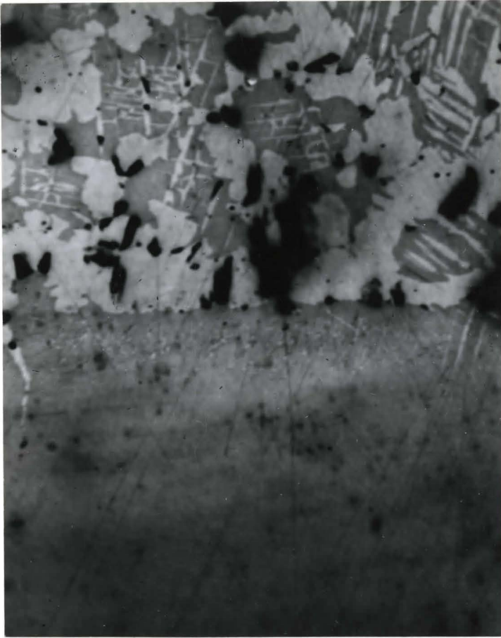
Figure 6.30 The interface of the FeS:MnS diffusion couple reacted at 1300°C for 15 minutes. X1120
