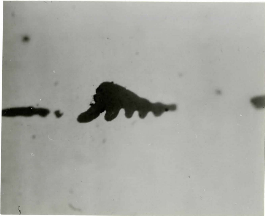
Figure 8.18 "Sinusoidal" Fe alloy/MnS inclusion interface caused during the FeS to MnS transformation. (courtesy of Hone (64) ) X800
