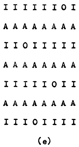
Figure 10. Schematic representation of order, and point and domain disorder, where I and O are two different cations.
