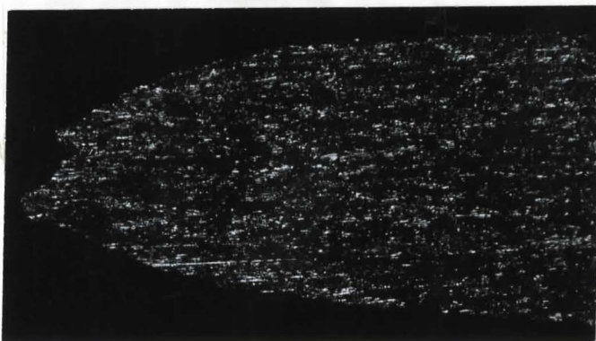
FIGURE 46 For Thickness Profile at Fracture Site Material 3003 - Aluminum Alloy, 66X
