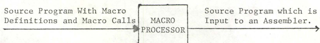
Fig. 1: Logical action of a Macro Processor
