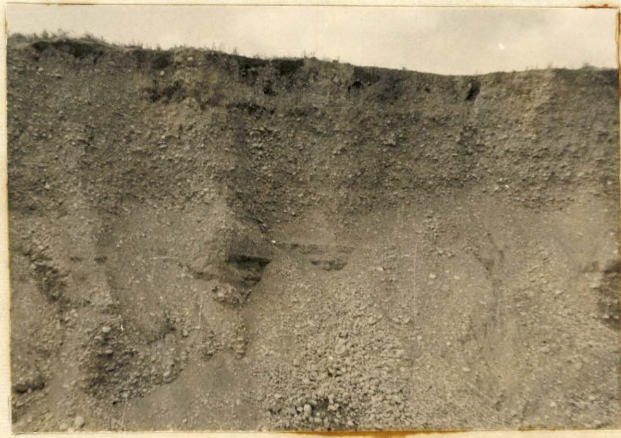
Fig. 3. A spillway gravel pit from which road materials are being taken. Quarrying as a commercial enterprise is of minor significance.
