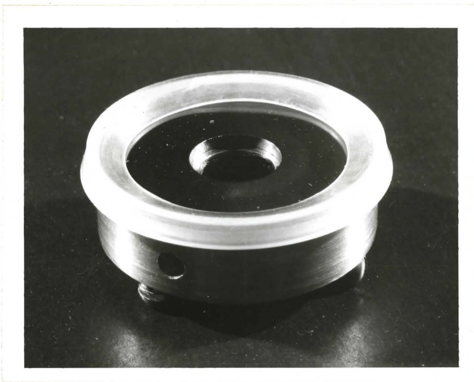
Figure 9. ^{210}\text{Po} source in holder (Source II)
