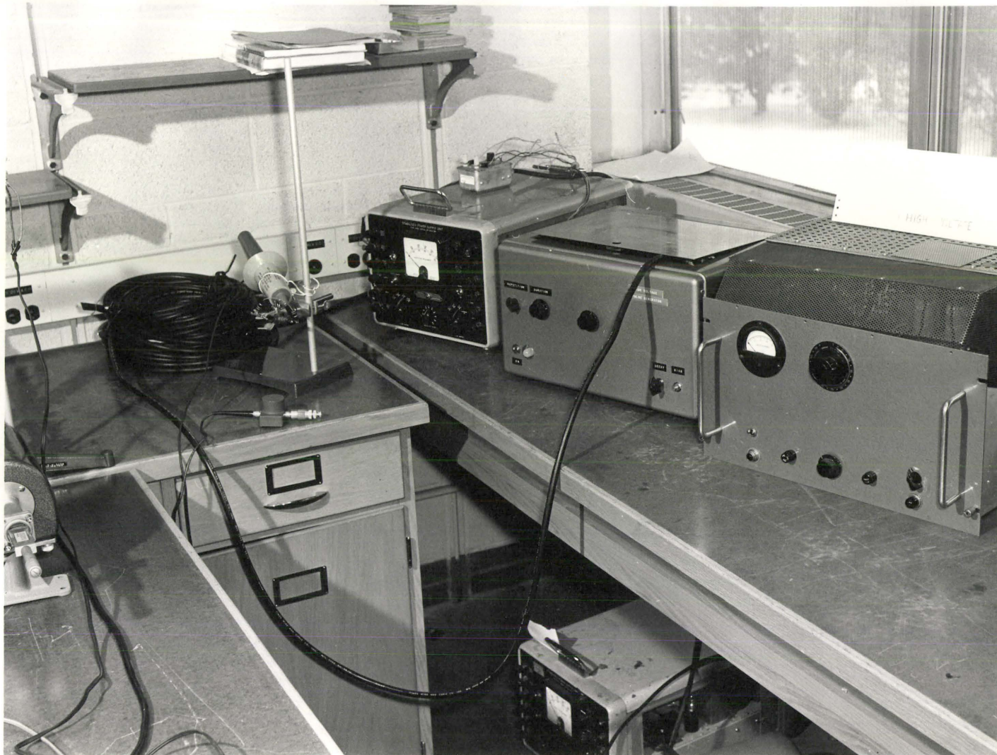
PHOTOGRAPH 2: The Pulse Generator; the Power Supply to the Pulse Generator and the High Voltage Supply.
