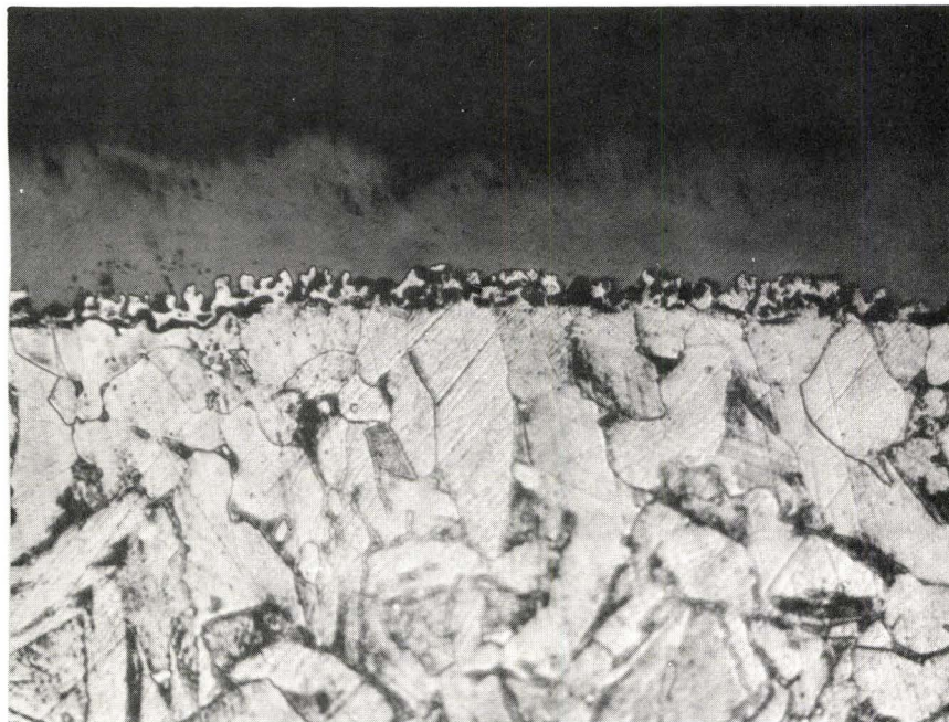
Figure 4-17 Void Formation and Iron Precipitation at Metal-Oxide Interface After Vacuum Decarburization for 3 hr. Void fraction at metal-oxide interface is 39%. x 400
