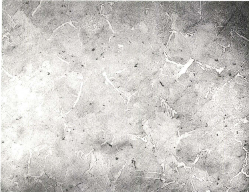
Figure 4-25 Incipient Decarburization at Center of Specimen. x 150
