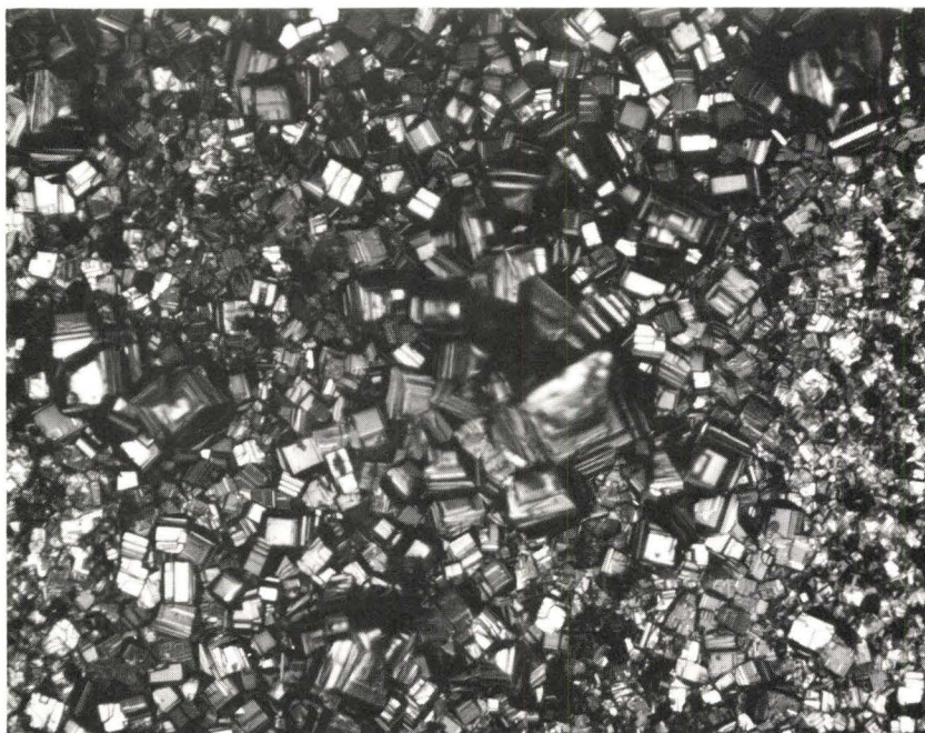
Figure 4-10 Surface Topography, Oxidation Time in \text{CO}_2 18 min. x 150
