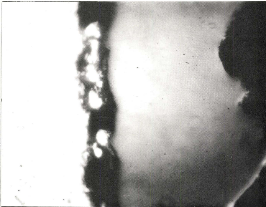
Figure 4-15 Void Formation and Iron Precipitation at Metal-Oxide Interface After Oxidation in \text{CO}_2 (unetched). x 380
