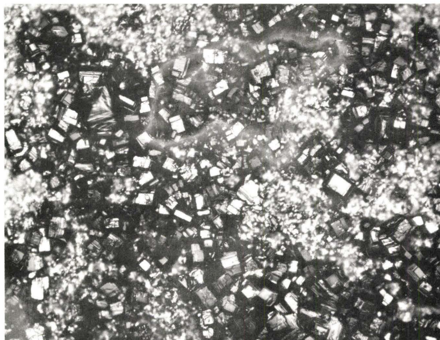
Figure 4-13 Surface Topography, Oxidation Time in \text{CO}_2 23 min., Vacuum Decarburization Time 141 min. x 150. Light areas indicate reduction of oxide to metal.
