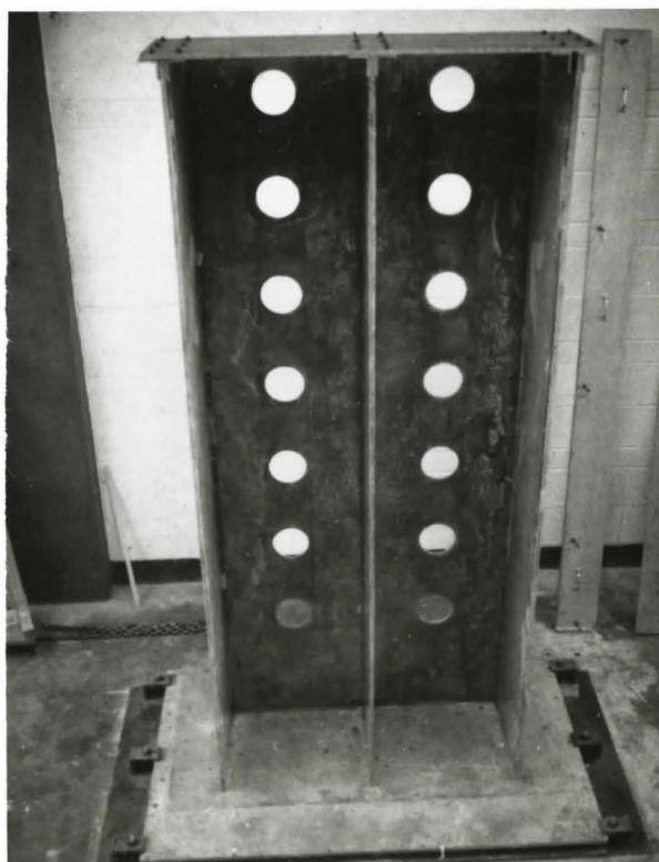
Fig. 3b Photograph of Model I Showing the Position of the Openings
