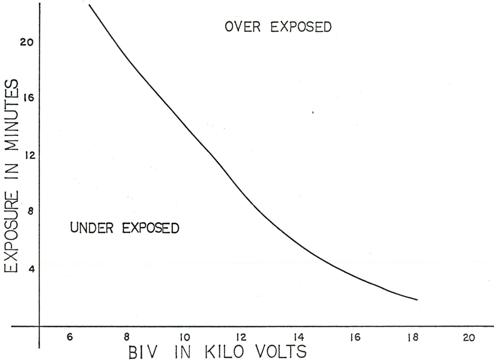
Figure 4.6 An empirical plot of the photographic exposure time versus the best image voltage.
