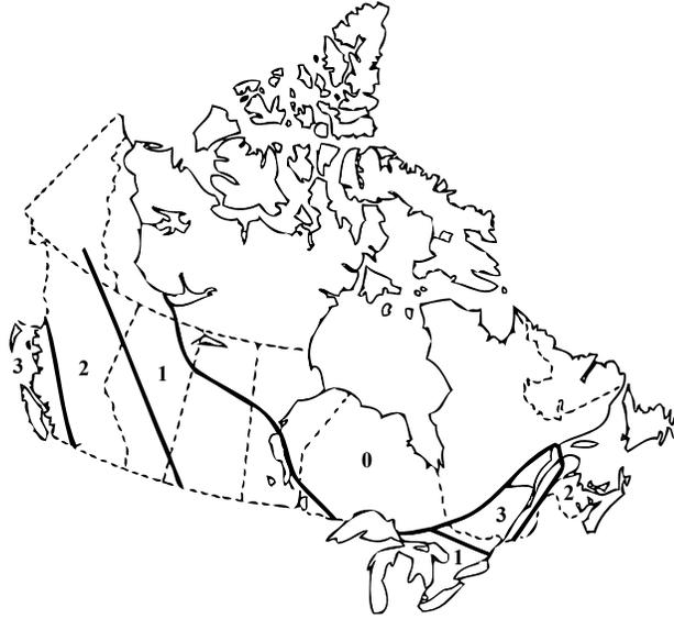
**Figure 5.2:** Seismic zoning map in the 1965 National Building Code of Canada [15]
