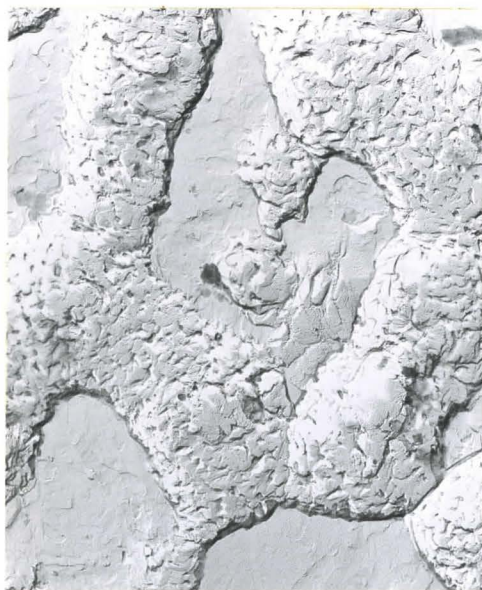
Fig. 33: A replica of the surface of a 7000Å NiO film form- ed at 600°C. x8000
