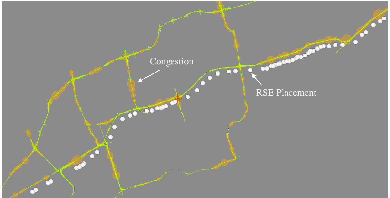
Figure 3.5: Traffic Conditions and Locations for RSE Placement
