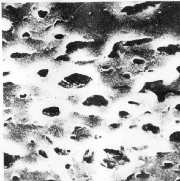
Figure (3-4-a) A scanning electron micrograph of unused Batch 2 charcoal, 1000x.
