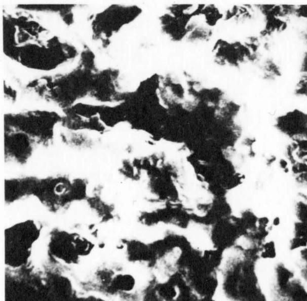
Figure (3-4-b) A scanning electron micrograph of used Batch 2 charcoal, 1000x.
