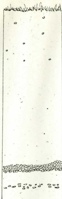
Fig. 5-10 Generalised profile of a Brighton sandy loam, the soil type typical of terrain type IV.
