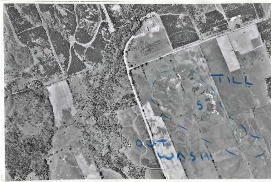
Photo. 5-42 Air photo representation of the slopes (s) which develop at the junction of till and outwash sands & gravels.
