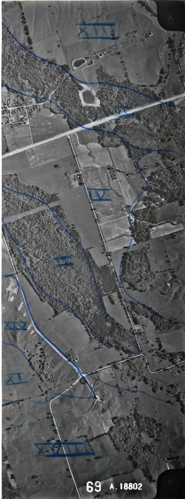
Photo. 4-1 An aerial photograph on which areas of characteristic pattern and tone have been outlined.
