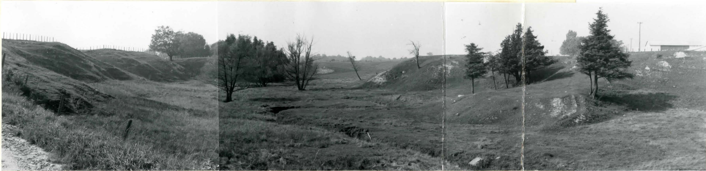
Photo.5-23 Illustrating ground conditions within a Linear Deposit of Alluvial Origin or Valley Flood Plain. Note drainage and secondary incision. Valley sides are composed of till and are subject to creep and local sod removal.
