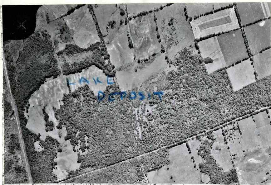
Photo. 5-14 Illustrating the air photo pattern which frequently characterises the Schomberg lake deposits.
