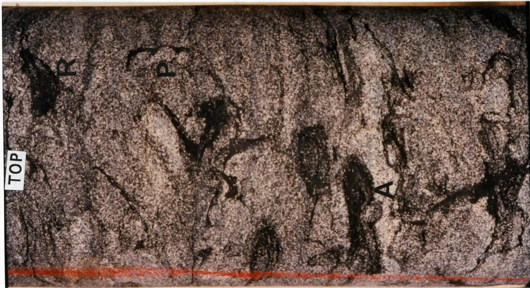
**Fig. 27.** Basal sandstones of Facies 3b completely bioturbated by *Rosselia*(R), *Asterosoma* (A) and *Paleophycus* (P). Well 5-8-54-19W5 depth 2556 m, 3" core diameter.
