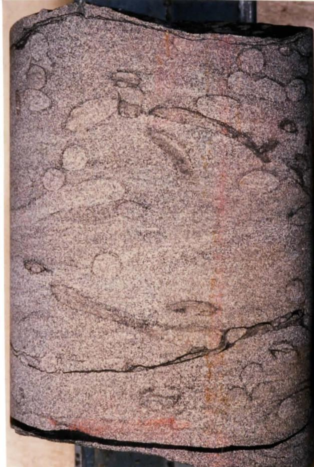
**Fig. 32.** Fine-grained sandstones of Facies 5a abundantly bioturbated by traces of *Paleophycus*. Well 3-24-57-19W5 depth 2642 m, 4" core diameter.
