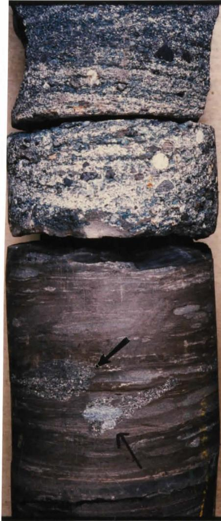
**Fig. 35.** The basal contact of Channel 6 is defined in this case by black mudstones of the Gething Formation (below) abruptly overlain by a glauconite rich pebbly sandstones representing a transgressive lag. *Thalassinoides* traces of the Glossifungites Ichnofacies are present within the mudstones (black arrows). Well 10-1-56-19W5 depth 2569 m, 3" core diameter.
