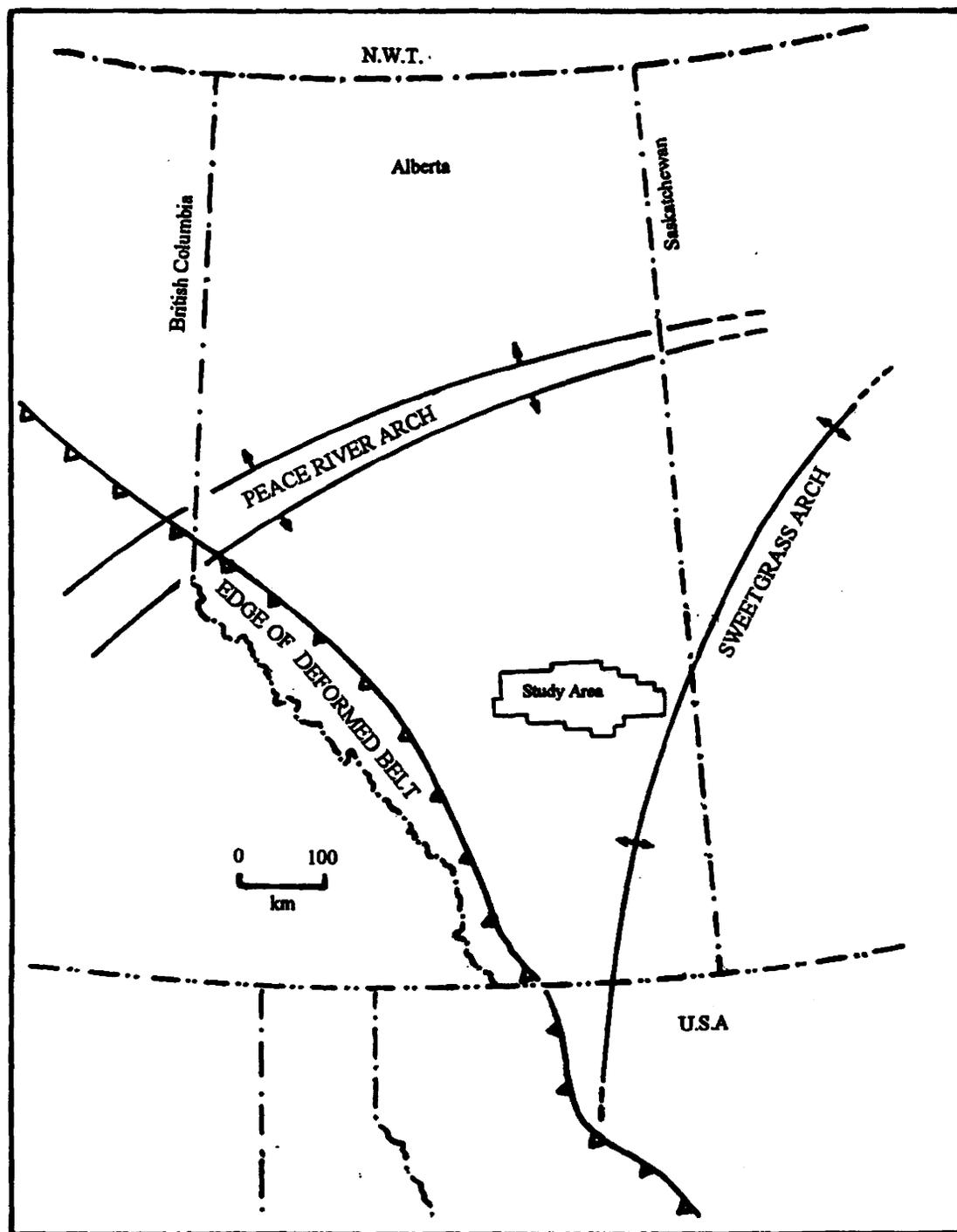
Figure 2.3 Major structural elements of the Western Canada Sedimentary Basin in comparison with study area location. (Modified from Wiseman, 1994)
