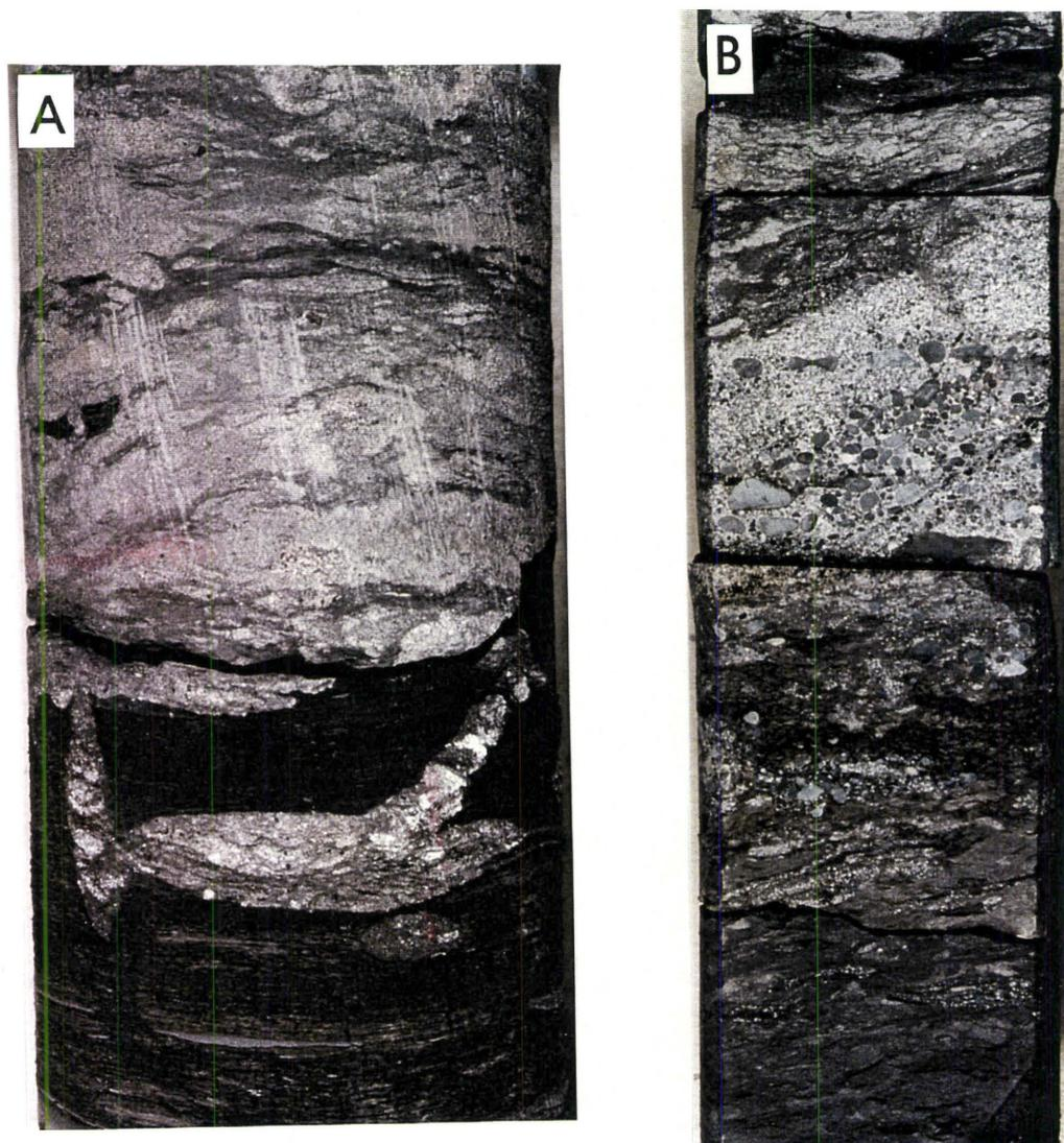
**Figure 4.8** A) BD1 at Hamilton Lake. Note the sharp contact with underlying mudstones of RV2 and prominent *Glossifungites* burrow (*Thalassinoides*?) subtending this surface (3" core from 4-17-35-7w4; 865.5 m). B) BD1 at Fenn West. Note the conglomeratic transgressive lag resting on this surface and the granules and coarse sand which are burrowed into underlying 'regional Viking' mudstones (3" core from 4-32-36-21w4; 4401').
