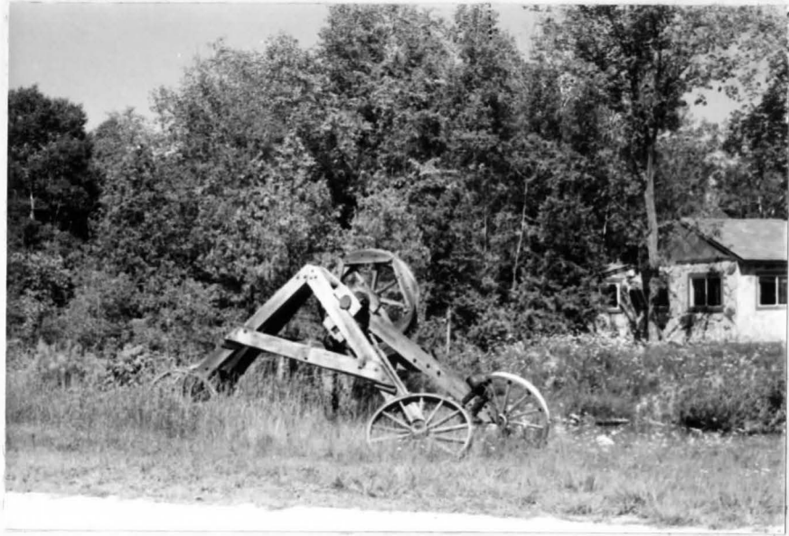
Illus. 11 Owing to the rocky nature of the land, one of the most important tools or machines in early days was the stone-puller. The boulder was raised slightly in the middle and then the whole machine was pulled by oxen or horses.
