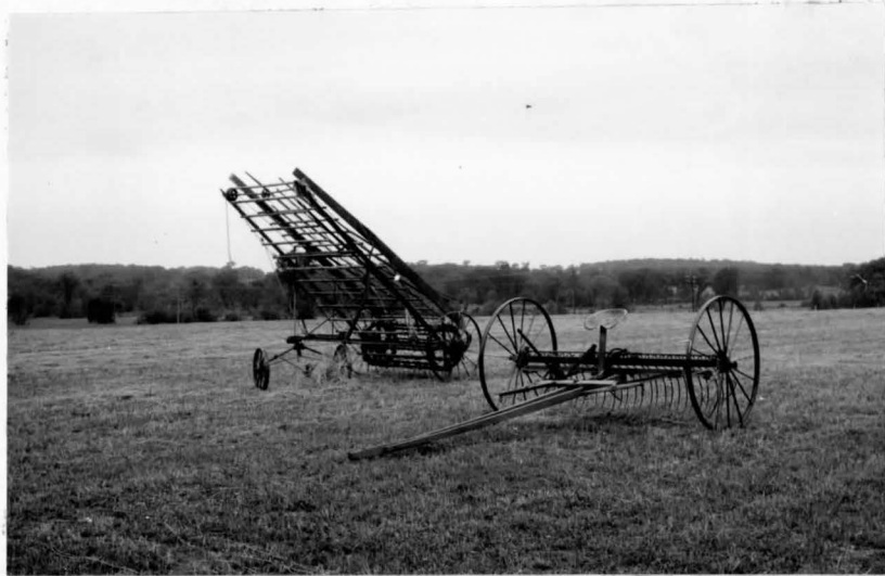
Illus. 23 The hay loader is still a very important piece of farm machinery in Keppel; but this style of rake has been largely replaced by the side delivery model.
