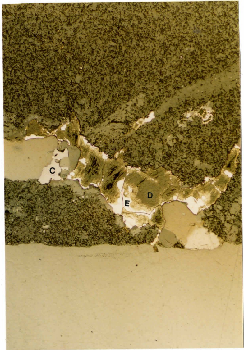
PLATE 3.13: Fracture controlled sphalerite (C) and pyrrhotite core (D) with possible Ni-rich corona (E). From M-320 under reflected (64x).
