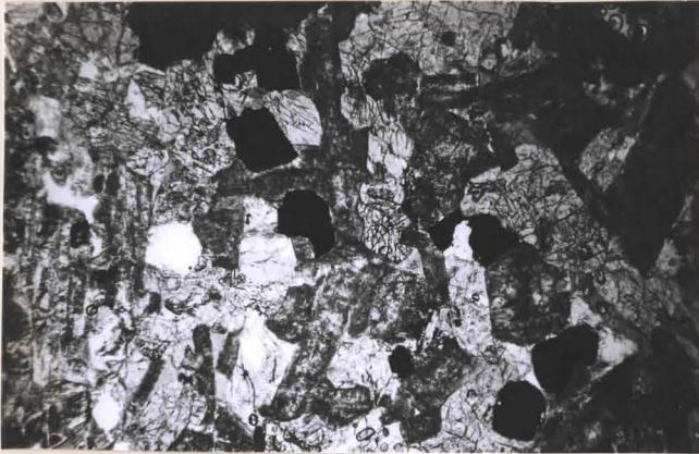
Fig. 28. Photomicrograph: cumulus magnetite in gabbro. Centre Hill. X 45
