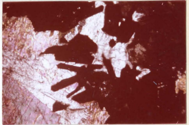
Fig. 10. Photomicrograph: clinopyroxene-hydrogrossular assemblage. Hydrogrossular black. Crossed nicols. X 45
