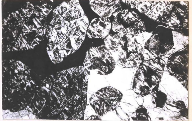
Fig. 3. Photomicrograph: poikilitic peridotite. Crossed nicols; clinopyroxene-light grey, altered plagioclase-dark. X 45
