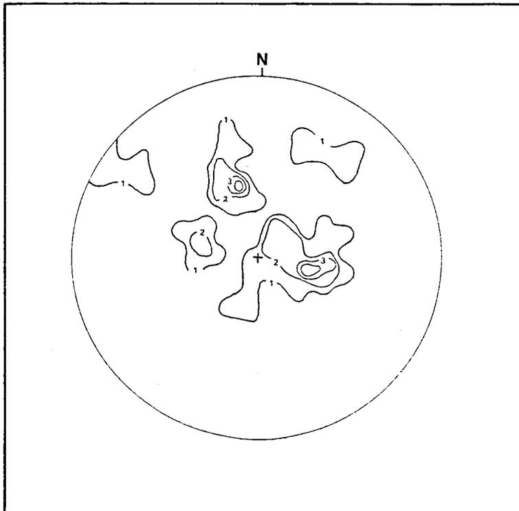
Figure 7.6 Contoured poles to the AB plane of clasts from station 3 (n = 20). Contours in increments of 1.
