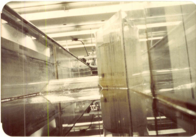
Fig. A1.5 - Flume Contraction (taken from inside the flume)
