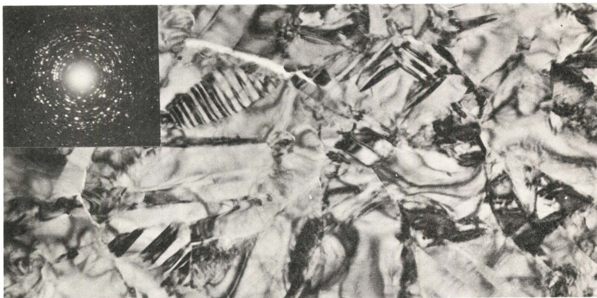
Fig. 5.7 ZrO_2 , mainly in the monoclinic form, produced by strongly pulse-heating an area similar to that shown in Fig. 5.6. Note the characteristic twinning. The inset shows the corresponding diffraction pattern.
