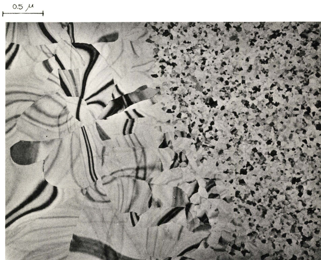
Fig. 6.7 Detailed view of interface between shadowed (left) and exposed (right) portions of an amorphous ZrO_2 film. The specimen was bombarded with 6 \times 10^{14} ions/cm 2 of 20-KeV Kr at a current of 20 \mu A/cm^2 . Note the occurrence of ordinary thermal crystallization, similar to Fig. (5.6), in the shadowed portion.
