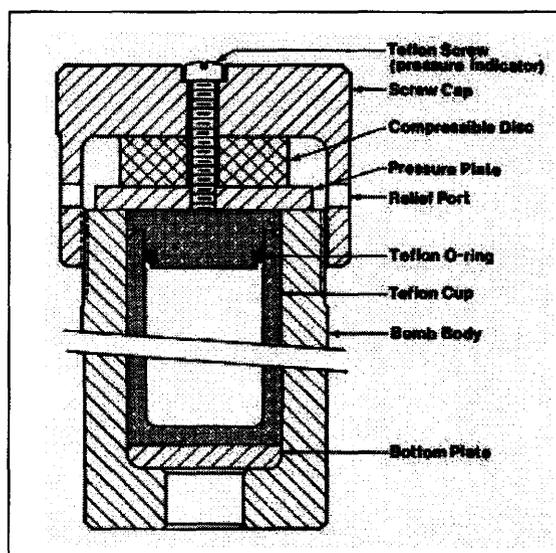
Figure 3.1: Schematic diagram of the Parr Microwave Acid Digestion Bomb.<sup>18</sup>
