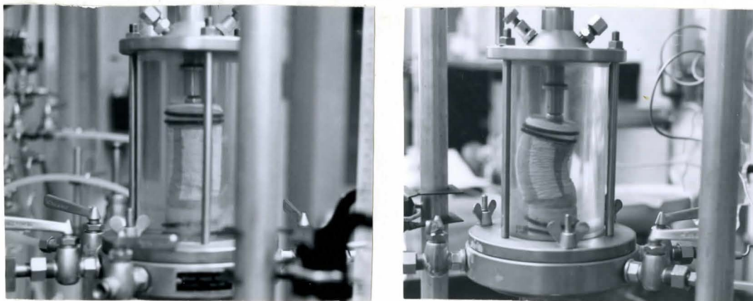
Fig. 4 - Typical Eccentric Sample Before and After Shearing Stage.
