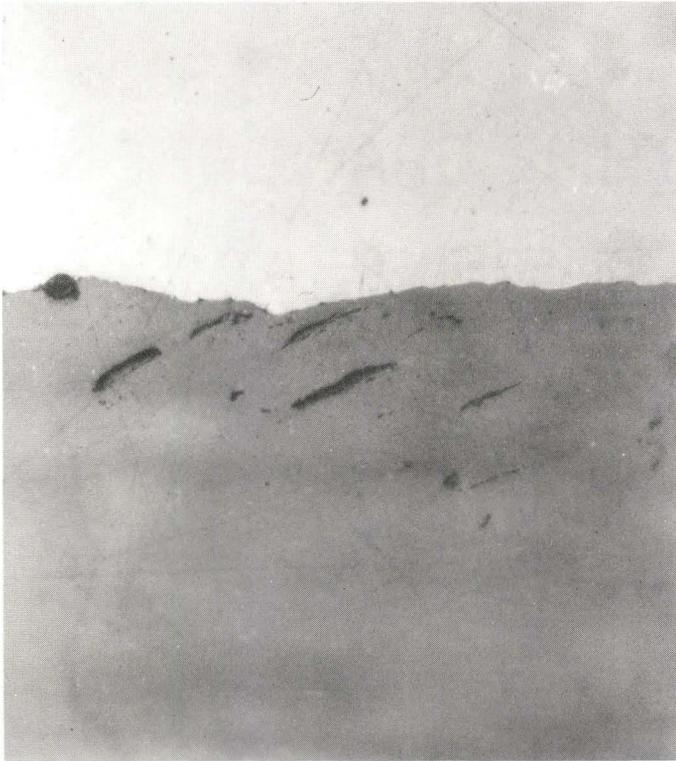
Fig. 23 Photomicrograph of the planar interface of the Fe vs. MnS couple diffused for 8 hrs. x 400
