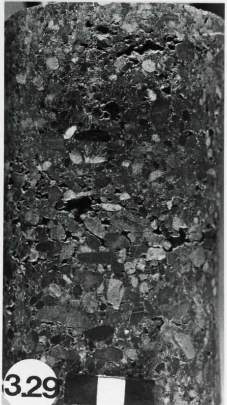
The conglomerates are mainly polymictic, clast supported and poorly sorted. The matrix is a lower to upper medium sand size, having a salt and pepper appearance similar to that in Facies E (Figure 3.28). There is no imbrication, nor any visible stratification. The pebbles lie both vertically and inclined. The clasts range in color from dirty-yellow, bluish-grey to black. The clasts are well-rounded and the larger ones (generally larger than 10 mm) are oblong in shape (Figure 3.29).
