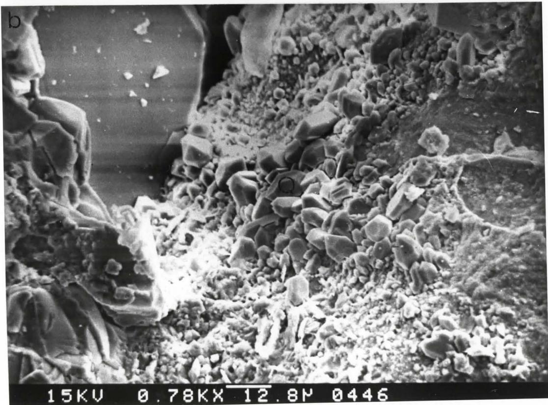
Fig. 4.16a, b and c. Scanning electron photomicrographs of progressively increased magnification (black outlined area) of a massive pebbly sandstone (Facies H). Note the authigenic quartz (Q) kaolinite booklets (K) in Figure 4.16c. Scale bar (microns) and magnification are located at the bottom of each photo, Figure 4.16c, 10-32-41-4W5, 6441 ft (1963.2 m).
