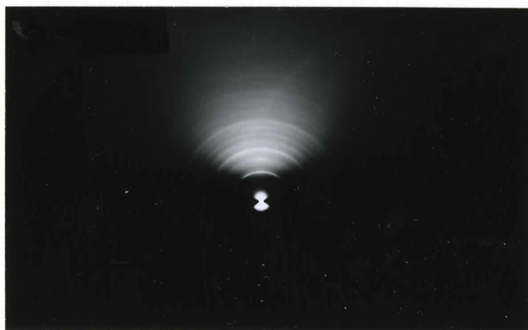
Figure 8-30 Reflection-electron-diffraction of (a) anodic \text{Nb}_2\text{O}_5 bombarded at 200^\circ\text{C} with 64 \times 10^{15} ions/ \text{cm}^2 , (b) anodic \text{WO}_3 bombarded at 200^\circ\text{C} with 12 \times 10^{15} ions/ \text{cm}^2 , and (c) anodic \text{WO}_3 bombarded at 200^\circ\text{C} with 24 \times 10^{15} ions/ \text{cm}^2 .
