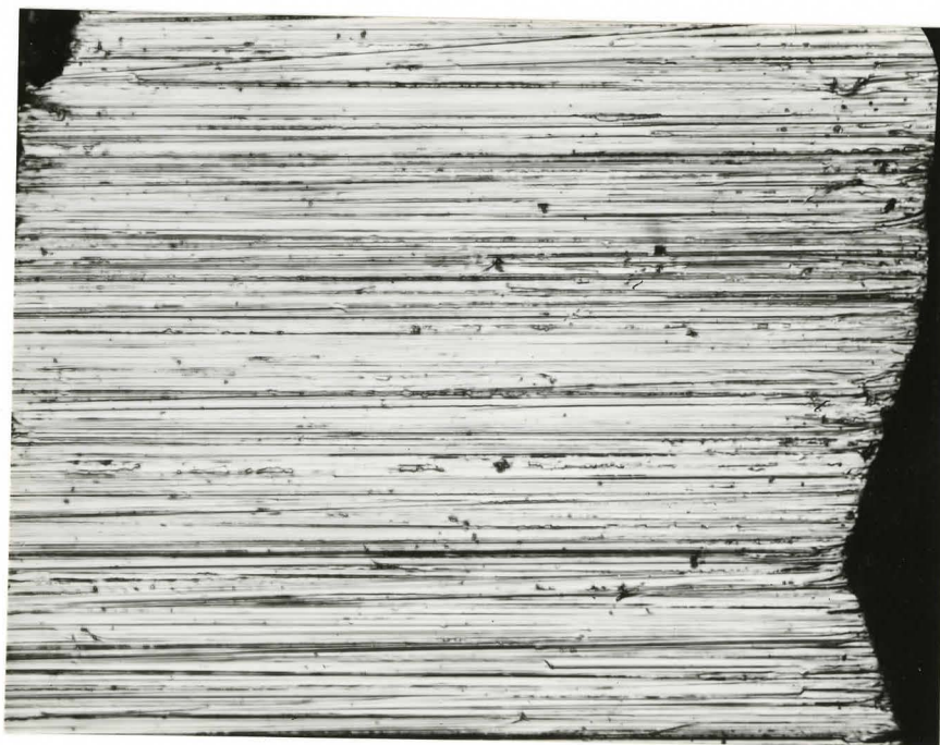
Fig.35. Wustite polished on 600 grit SiC using kerosene as lubricant. 300X
