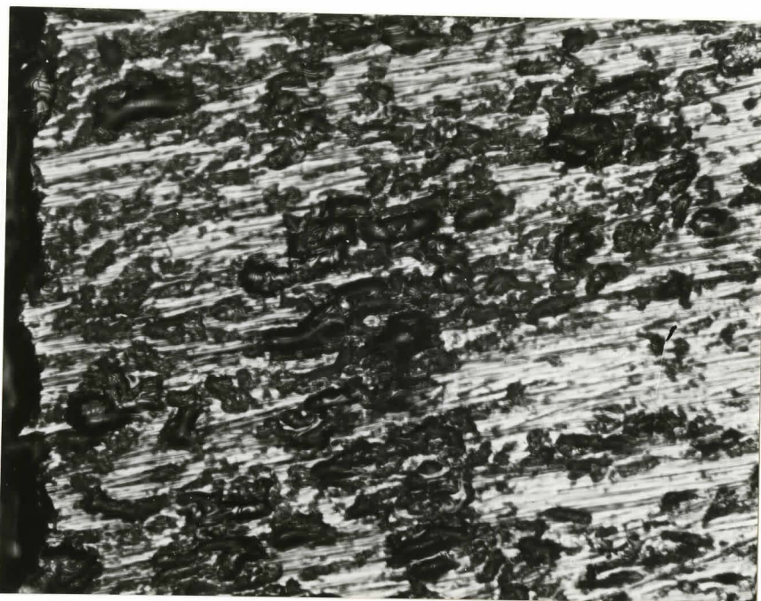
Fig.34. Wustite polished on 600 grit SiC using H_2O as lubricant. 300X
