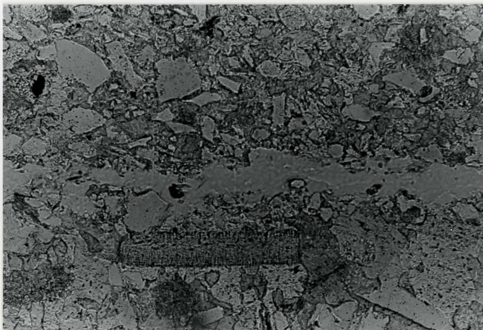
Photo 20: Burrows in Canada Brick Streetsville limestone. Scale: .5 mm across long axis.
