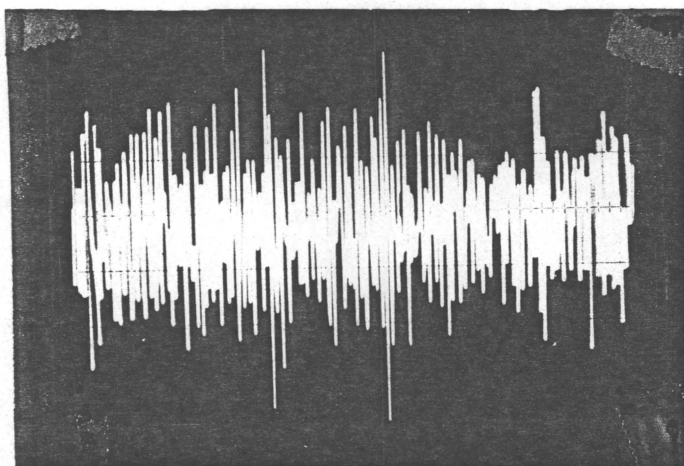
Fig. 5.64 A picture of 40ms pulsed CW signal at 512.5 Hz embedded in noise
