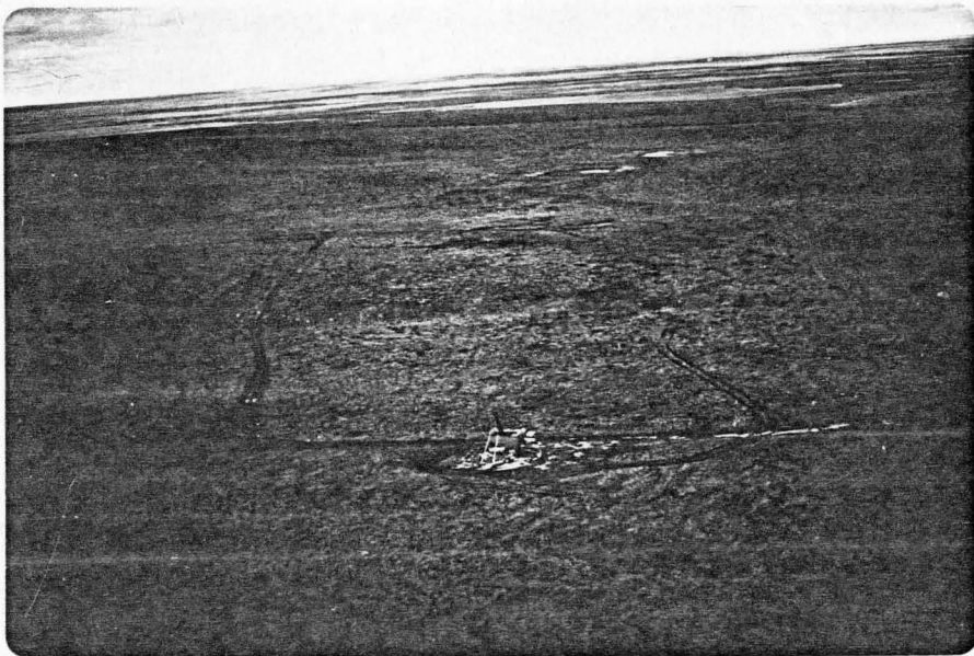
Figure 5.2 Aerial view of the differences in tracked vehicle and drill disturbances between thick peat areas (foreground) and areas of thin vegetation cover (background).
