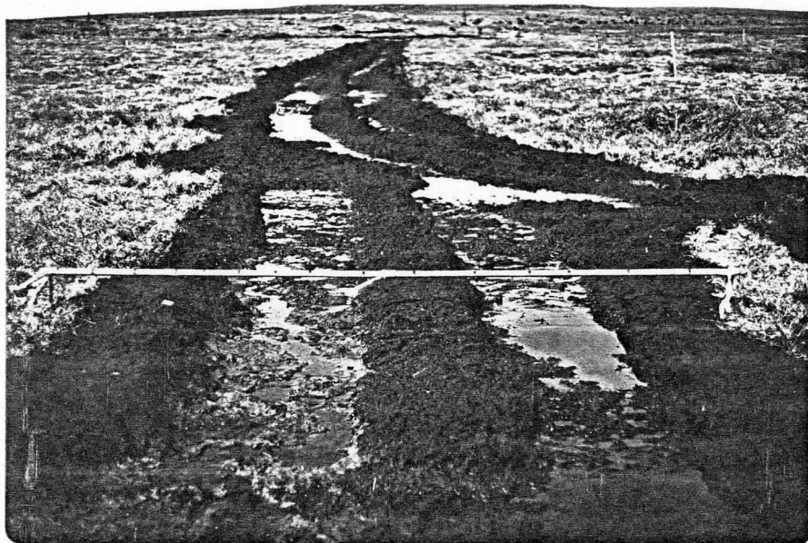
Figure 4.2 Bedstead 1, June 11. The slurried peat has formed after approximately 35 vehicle passes between late May and early June.
