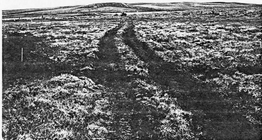
Figure 4.11 Main track 2 in early August where it crosses upper sedge meadow. Use of this track began in early July when thaw was well advanced. Rutting and slurring is considerably less advanced than for MT 1.
