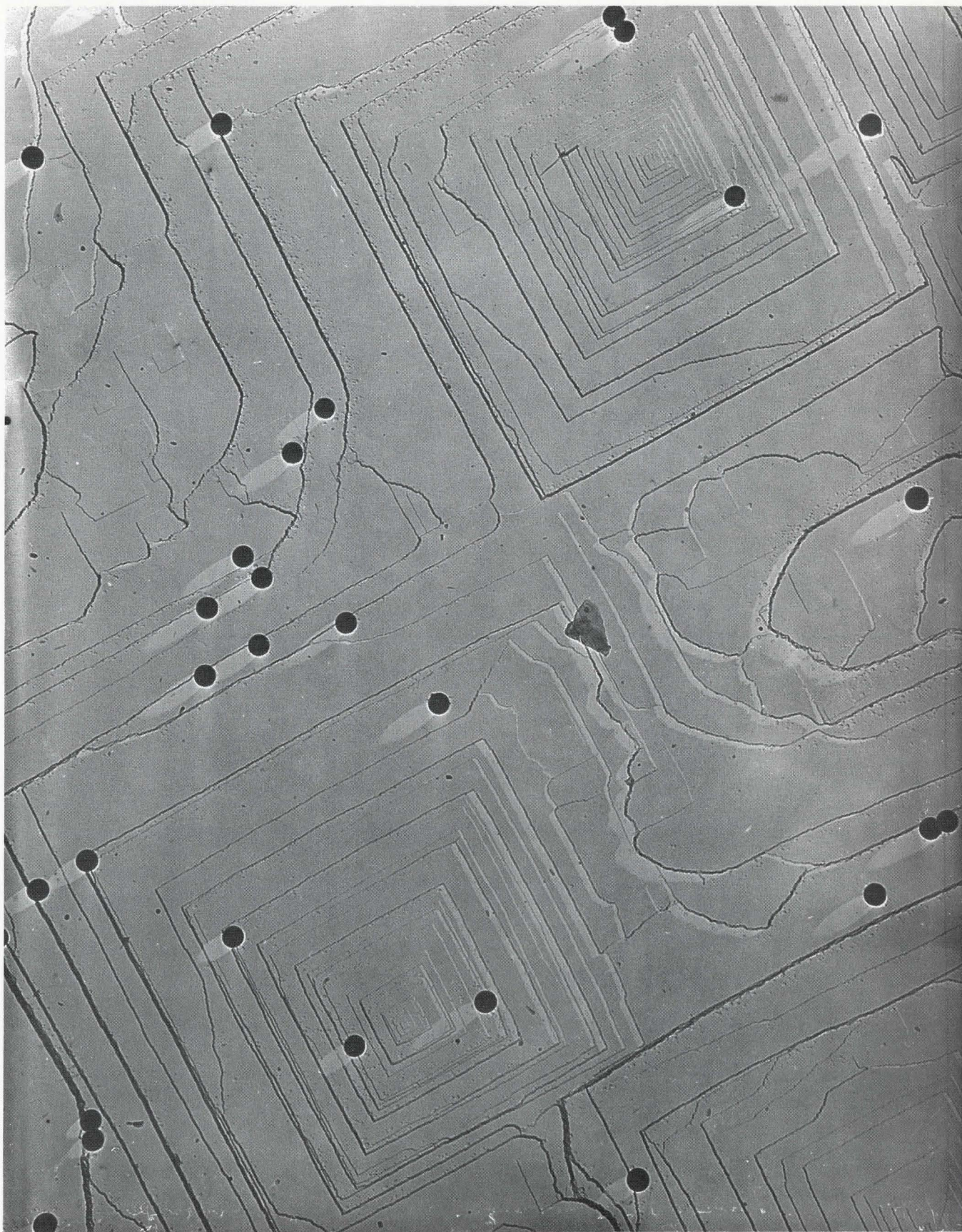
Figure 26: 2 minute, 10 ppm \text{Fe}^{+3} gel etch. (11,000 X)
