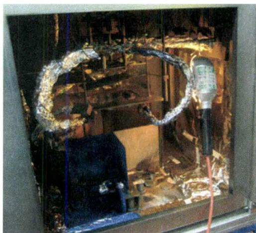
Figure 2.4: Thermal evaporator used for vacuum processing
