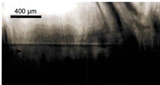
Figure 4.27: Optical micrograph of permanent conical structures formed after A) dark diffraction rings and B) bright diffraction rings in the right hand side and their corresponding intensity profiles in the left hand side for a sample ( \text{OPL} = 8.82 \text{ mm} ) with 1.6 \text{ W/cm}^2 of input beam intensity. For comparison, the permanent waveguide structure induced by a self-trapped beam is shown (C). The propagation direction of the beam ( z ) is indicated. (In order to best visualize the structures, micrographs in (A) and (B) were acquired with the sample placed at an angle. The scale bar is therefore approximate).
