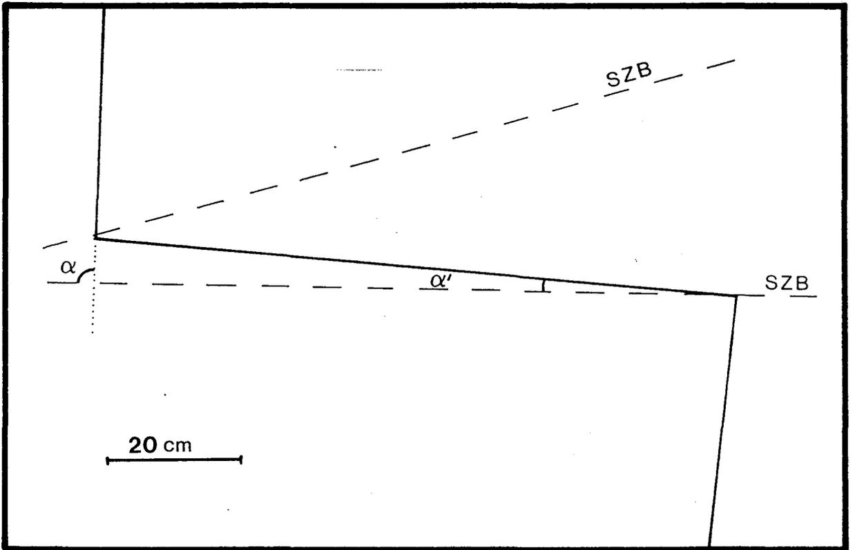
Figure 15. Shear strain construction from a pegmatite dyke which has been brittlely offset along several microfaults (taken from plate 6 in text).
