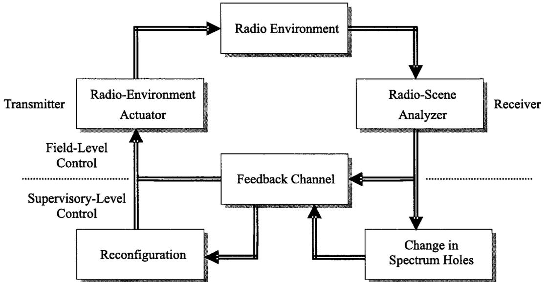
Figure 8.3: Two-level control scheme for cognitive radio.
