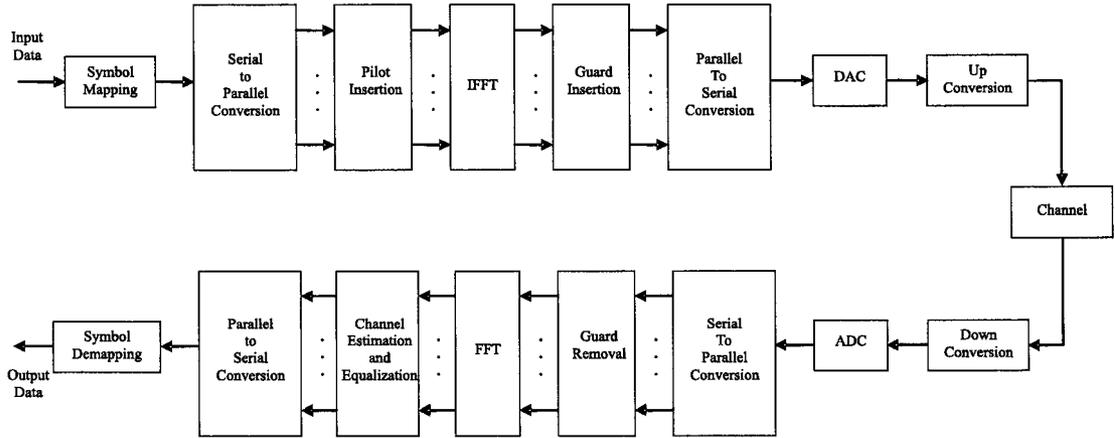
Figure 2.1: Block diagram of an OFDM transceiver.
