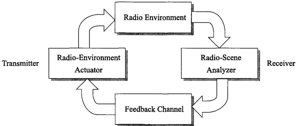
Figure 2.3: The cognitive-information-processing cycle in cognitive radio.
