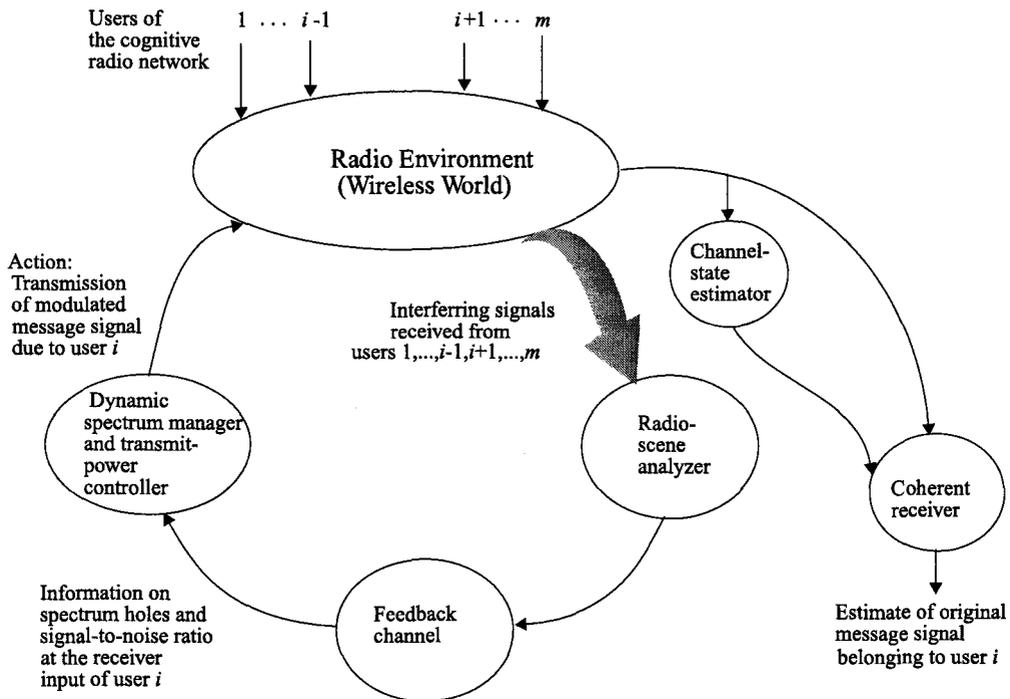
Figure 2.2: Basic information-processing cycle for user  $i$  in a cognitive radio network [1].
