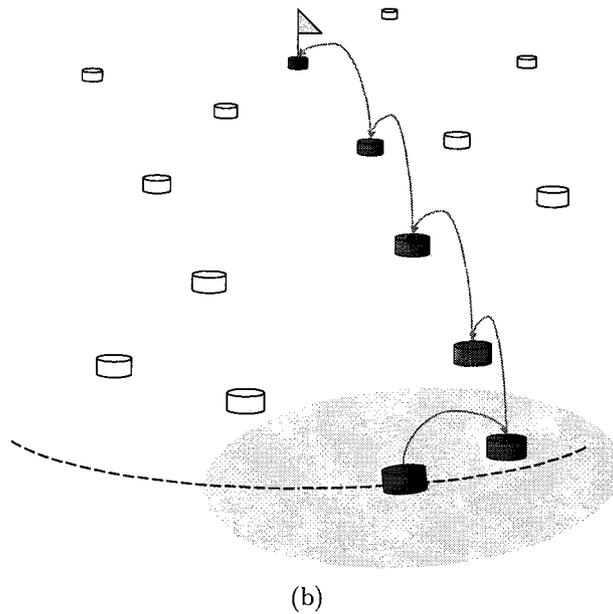
Figure 5.2: Effect of user mobility on the communication path: (a) partially changed, (b) completely changed.
