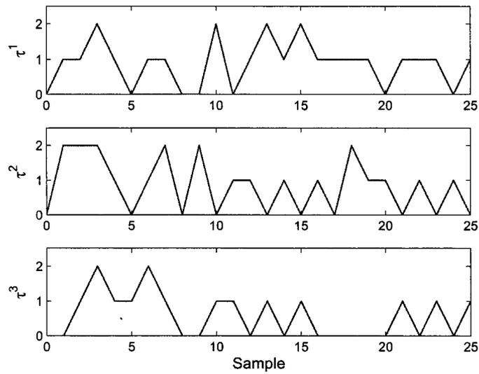
Figure 7.4: Time-varying delays introduced by feedback channels in transmit power control loops for a network of 3 users.
