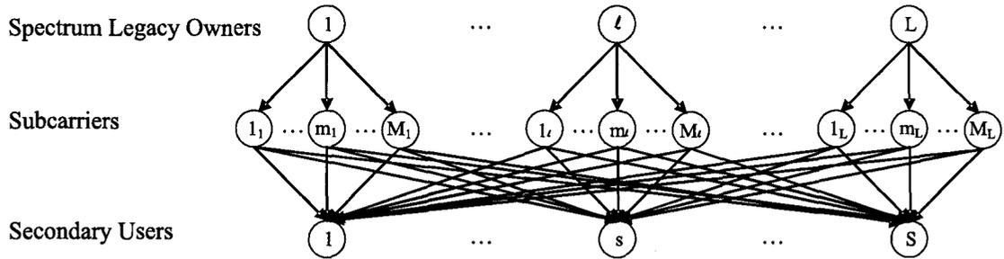
Figure 8.1: The spectrum supply chain network.
