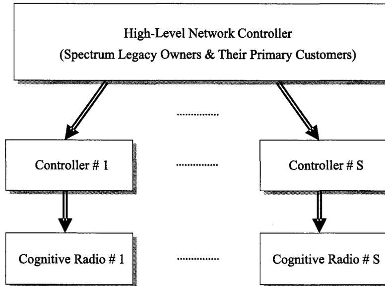
Figure 8.2: Decentralized hierarchical control structure in a cognitive radio network.
