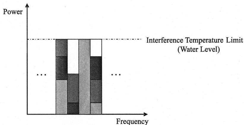
Figure 4.1: Waterfilling interpretation of the information-capacity theorem.
