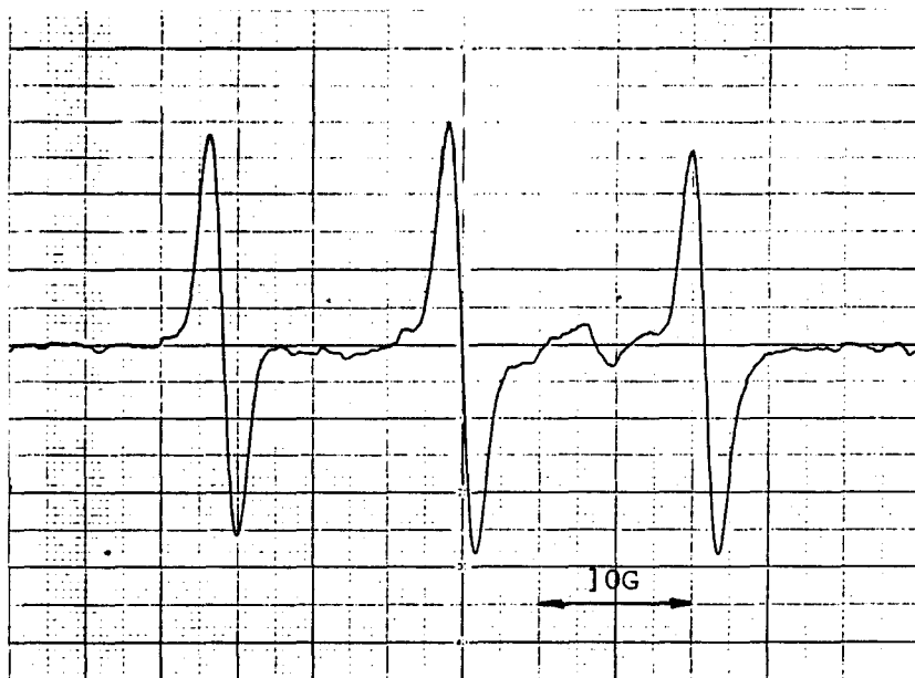
Figure 15: Ambient temperature e.s.r. spectrum after 10a irradiation at 120 K in an e.s.r. cavity and then warmed to ambient temperature.
