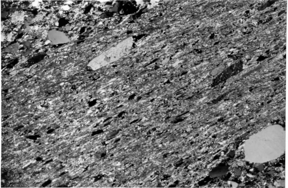
Figure 1.3.2 Slide G26-415BC. Rectangular quartz grain within a cleavage zone. The rectangular shape is due to unidirectional pressure solution. Note the mica beards at the ends of the grain. The grain is 0.5 mm.
