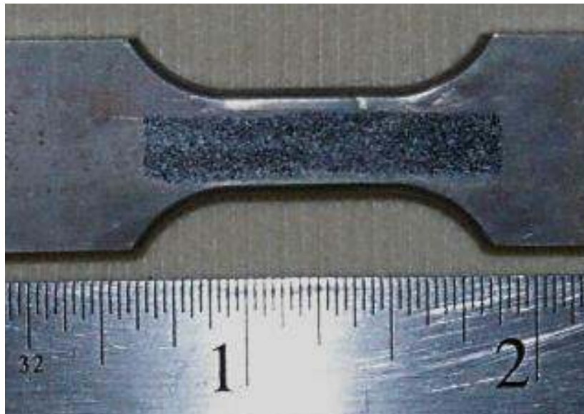
Figure 3.4: Drawing of stochastic mask on flat specimen used for global strain DIC
